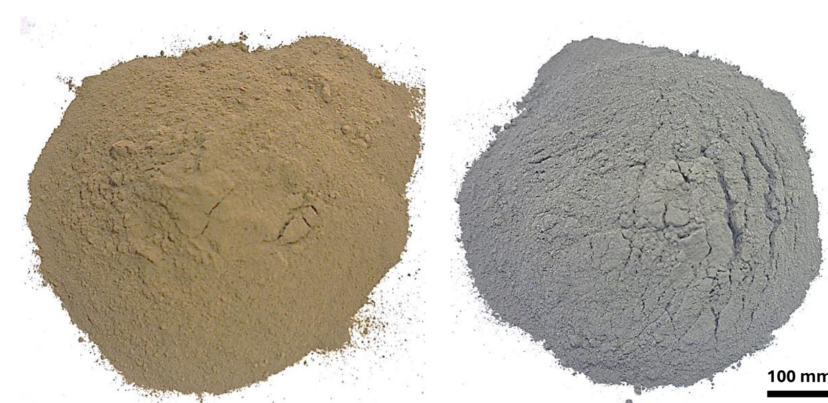
Figure 2. Two types of tailings material: brown, surface-derived and oxidized, and gray, unoxidized, from a drill core.
